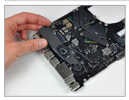
• Lift the left speaker assembly out of the logic board.
