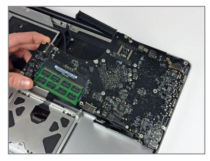
• Carefully lift the logic board assembly from the left side and work it out of the upper case, minding the port side that may get caught during removal.
