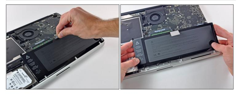
• Lift the battery by its plastic pull tab and slide it away from the long edge of the upper case.
