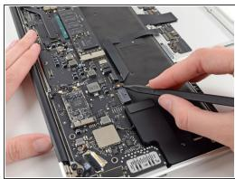
Use the tip of a spudger to flip up the retaining flap on the keyboard backlight ribbon cable ZIF socket.
