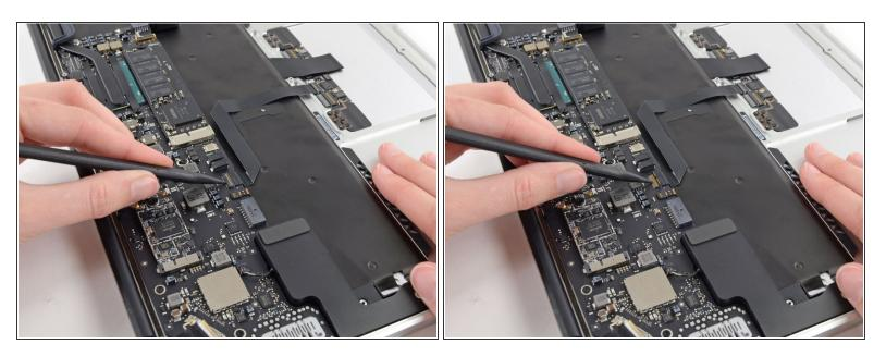
Use the tip of a spudger or your fingernail to flip up the retaining flap on the trackpad ribbon cable ZIF socket.
