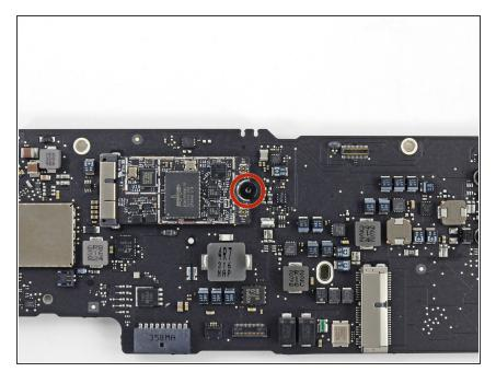
Remove the single 2.9 mm T5 Torx screw securing the AirPort/Bluetooth board to the logic board.
