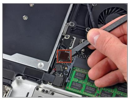
Use a spudger to pry the optical drive connector straight up off the logic board.
