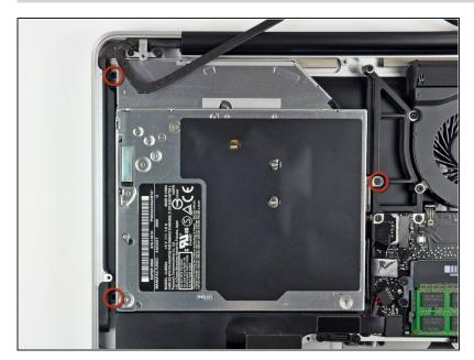
Remove three 3.5 mm Phillips screws securing the optical drive to the upper case.
