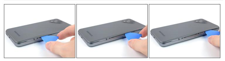
Using your thumbnail or an opening pick, slide along the right side of the phone to loosen the plastic clips.
