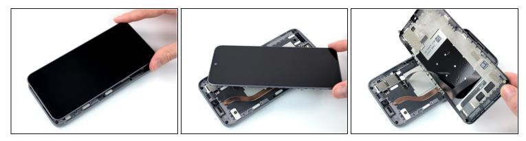
1 Do not remove the screen yet. It's still connected to the phone with a connection cable.
