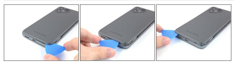
Slide along the bottom of the phone to loosen the plastic clips.
