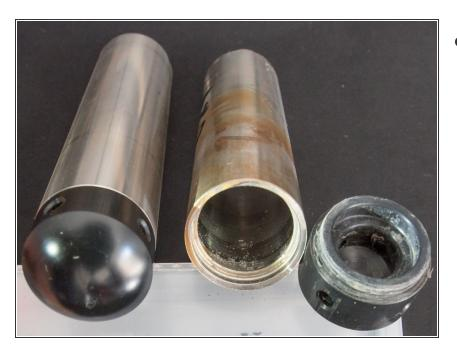
Remove the plastic end cap that protects the pressure and temperature sensor. The sensor is not attached to the end cap and it might be necessary to use quite a bit of force to get it off. I had to use vice grips and a bench vice for some loggers. You can also stick a screw driver through the holes and pull it off that way.
