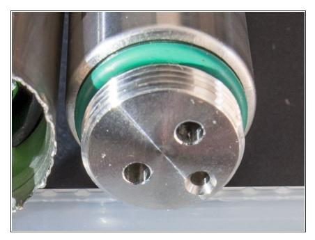
Remove the plastic screw on cap and remove the green O-ring.
