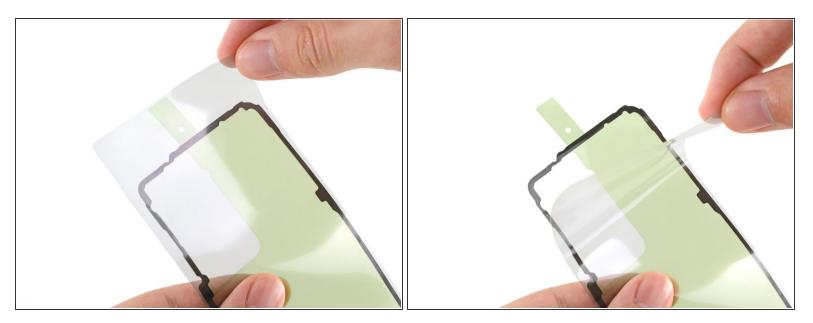
• Peel the **clear liner** off of the adhesive strip to expose the adhesive.
