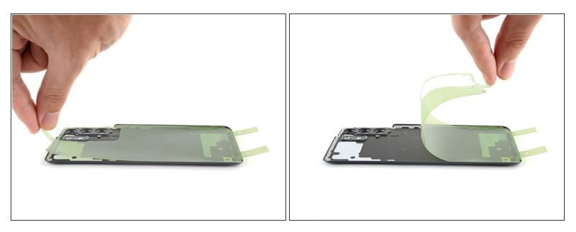
• Peel off the **colored liner** from the adhesive strip to expose the opposite side of the adhesive.
