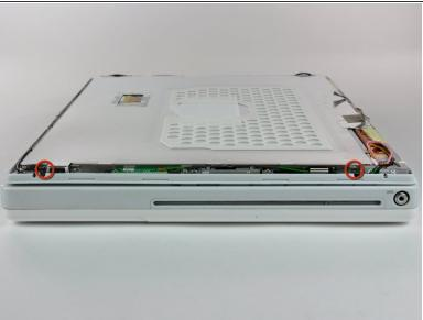
Remove the two Phillips screws securing the left and right sides of the LCD to the frame of the clutch hinges (four screws total).
