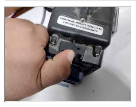
Secure the roller assembly cover to the pump by rotating the latch on the left side of the pump casing and using your thumb rotate it from the right fully to the left.
