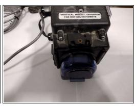
Locate the latch on the left side of the pump casing and using your thumb rotate it from the left fully to the right.
