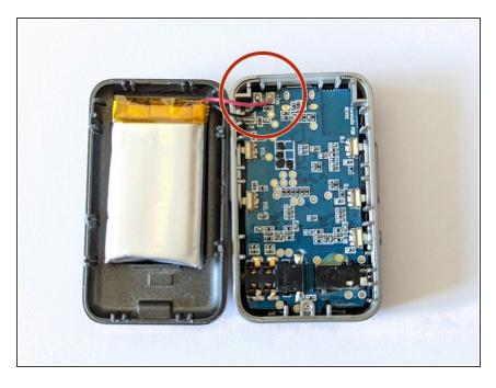
Flip the back panel aside the device.
