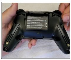
Place the battery into the socket by aligning the connectors on the battery with the connectors on the right of the battery socket.
