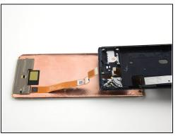
• Turn the phone over and remove the midframe while gently threading the screen ribbon cable through the opening in the midframe.
