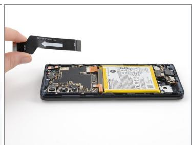
• Use your fingers to remove the interconnect cable after it has been disconnected from both the motherboard and daughterboard.
