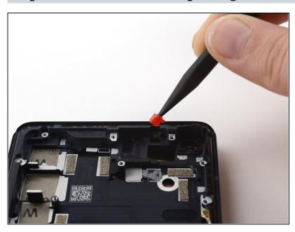
Use a spudger to dislodge and remove the red microphone gasket from the top of the midframe.
