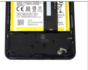
• Use a T5 Torx screwdriver to remove the nine 3.4 mm screws securing the daughterboard.
