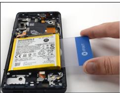
Carefully slide a plastic card underneath the battery to cut through the adhesive.
