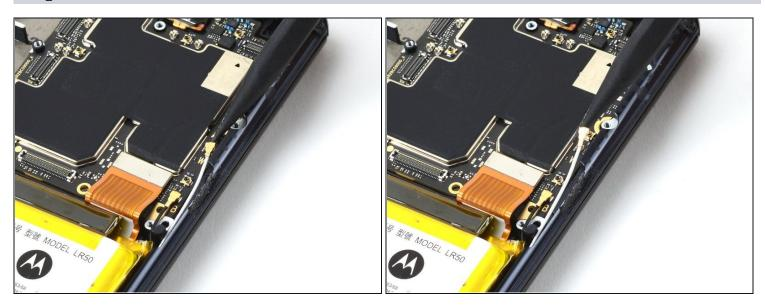
• Use a spudger to pry up the white coaxial cable and detach it from the motherboard.
