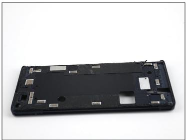
• Once the fingerprint sensor has been removed, the midframe is ready to be replaced.
