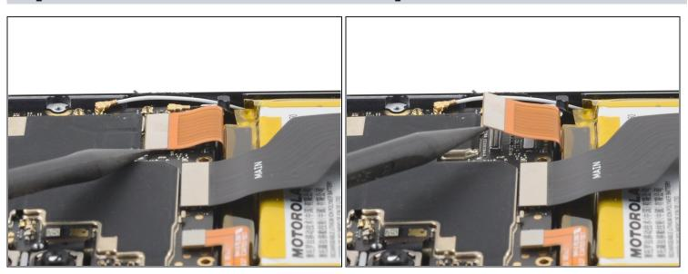
• Use a spudger to pry up and disconnect the screen ribbon cable's press connector from the motherboard.
