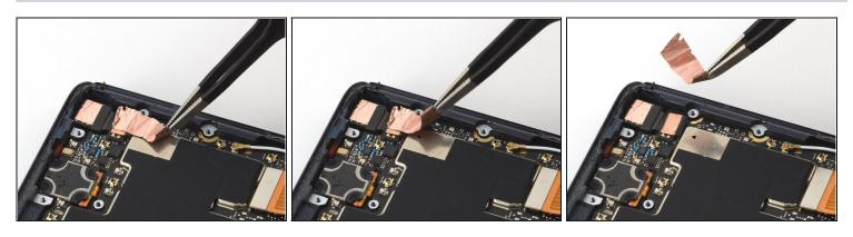
• Use a pair of blunt tweezers to peel up and remove the copper tape covering the front camera ribbon cable.
