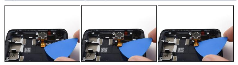
Use an opening pick to disconnect the earpiece speaker cable from the midframe.
