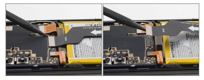
• Use a spudger to pry up and disconnect the interconnect cable's press connector from the motherboard.
