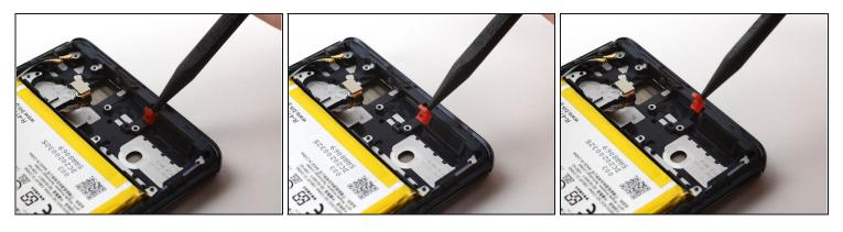
• Insert the pointed end of a spudger behind the microphone gasket at the bottom of the midframe.
