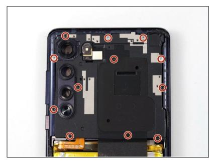
Use a T5 Torx screwdriver to remove the twelve 3.4 mm-long screws securing the motherboard cover.
