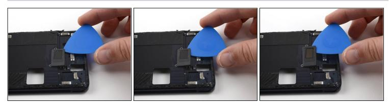
• Use an opening pick to carefully separate the fingerprint sensor cable from the midframe.
