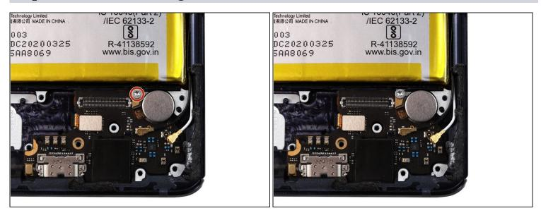
Use a T5 Torx screwdriver to remove the single 3.2 mm screw securing the daughterboard.
