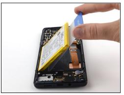
Slide a plastic card under the battery, then carefully lift the battery up until the adhesive is loose enough to remove the battery.
