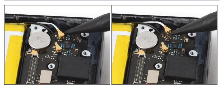
Use a spudger to pry up the white coaxial cable and disconnect it from the daughterboard.
