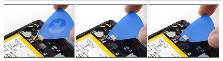
• Use an opening pick to carefully separate the vibrator's ribbon cable from the frame of the phone.
