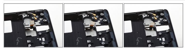
• Turn the phone over, then carefully thread the fingerprint sensor cable through the opening in the midframe.
