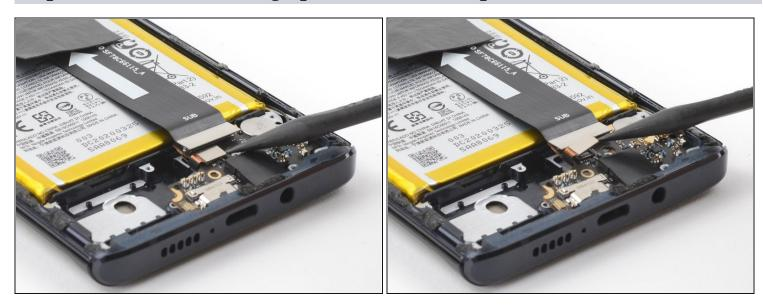
• Use a spudger to pry up the fingerprint sensor cable's press connector and disconnect it from the daughterboard.
