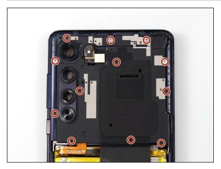
Use a T5 Torx screwdriver to remove the twelve 3.4 mm-long screws securing the motherboard cover.
