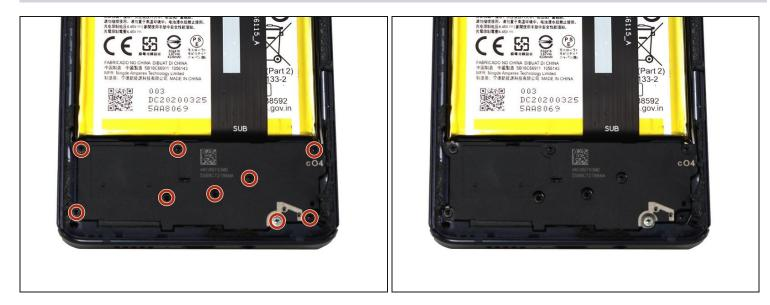
• Use a T5 Torx screwdriver to remove the nine 3.4 mm screws securing the daughterboard.
