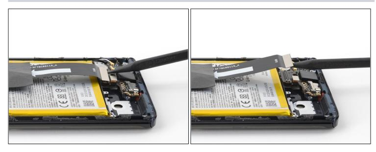
Use a spudger to pry up and disconnect the interconnect cable's press connector from the daughterboard.
