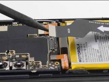
Use a spudger to pry up and disconnect the interconnect cable's press connector from the motherboard.
