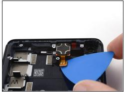
• Use an opening pick to disconnect the earpiece speaker cable from the midframe.
