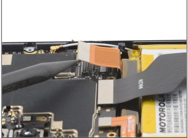
Use a spudger to pry up and disconnect the screen ribbon cable's press connector from the motherboard.
