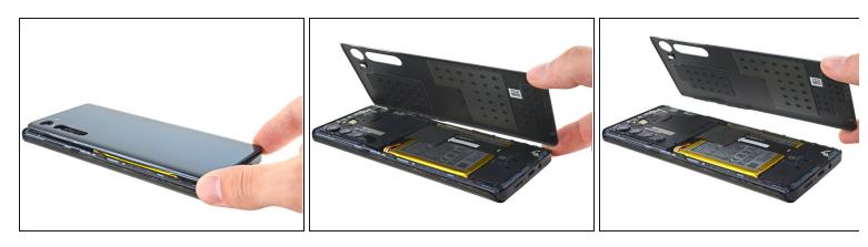
• Remove the back cover, taking care not to damage the components inside the phone.
