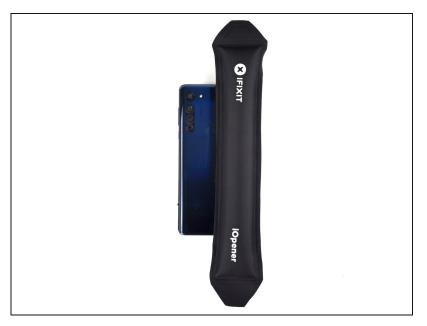
Apply a heated iOpener to the back cover's right edge for two minutes.
