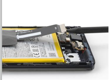
Use a spudger to pry up and disconnect the interconnect cable's press connector from the daughterboard.
