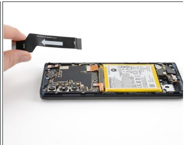
• Use your fingers to remove the interconnect cable after it has been disconnected from both the motherboard and daughterboard.
