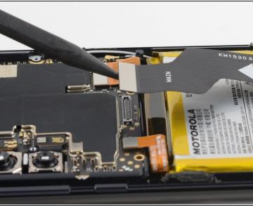
• Use a spudger to pry up and disconnect the interconnect cable's press connector from the motherboard.
