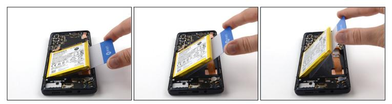
• Slide a plastic card under the battery, then carefully lift the battery up until the adhesive is loose enough to remove the battery.
