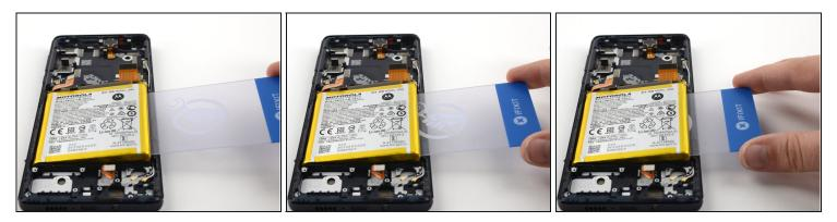
• Carefully slide a plastic card underneath the battery to cut through the adhesive.
