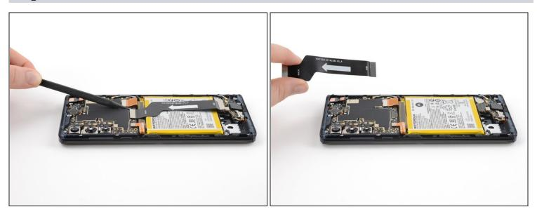
• Use your fingers to remove the interconnect cable after it has been disconnected from both the motherboard and daughterboard.
