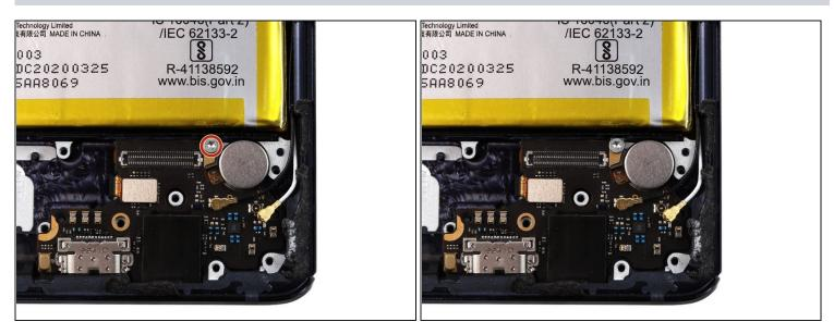
• Use a T5 Torx screwdriver to remove the single 3.2 mm screw securing the daughterboard.
