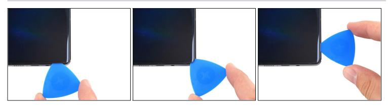
• Rotate the opening pick around the bottom-right corner of the phone.
