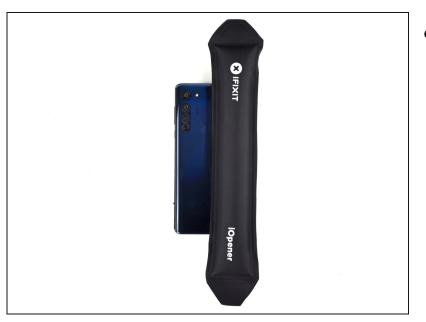
Apply a heated iOpener to the back cover's right edge for two minutes.
