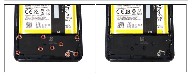
• Use a T5 Torx screwdriver to remove the nine 3.4 mm screws securing the daughterboard.
