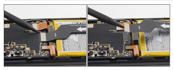
• Use a spudger to pry up and disconnect the interconnect cable's press connector from the motherboard.
