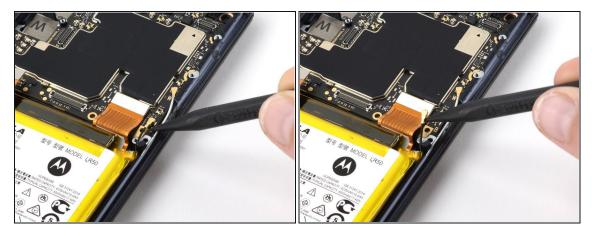
• Use a spudger to pry up the black coaxial cable and detach it from the motherboard.
