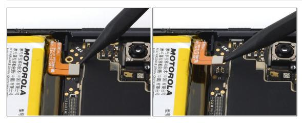
• Use a spudger to pry up and disconnect the battery cable's press connector from the motherboard.
