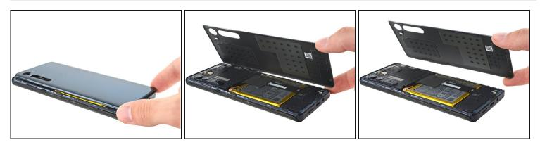
Remove the back cover, taking care not to damage the components inside the phone.
