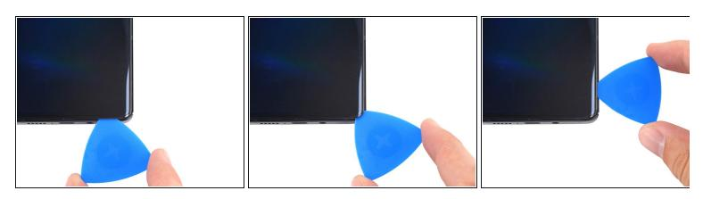
• Rotate the opening pick around the bottom-right corner of the phone.
