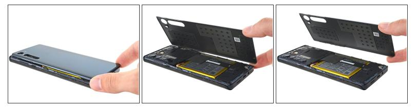
• Remove the back cover, taking care not to damage the components inside the phone.
