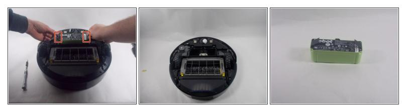
• Lift out the battery by pulling up on the two flexible tabs that are attached to the left and right sides.
