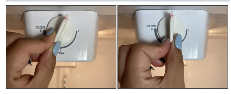
Set the temperature switch in the refrigerator to "OFF."
