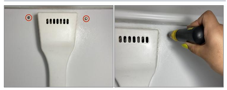
Use a 6 mm Allen key to remove the two 6.0 mm screws securing the freezer's interior back cover.
