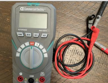
Turn the dial until the little green mark is set on the "OFF" option. Next disconnect the two testing leads by simply pulling them away from the body. Set these aside for later.
