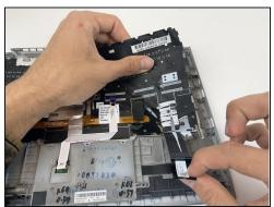
Carefully pull back on the black tab to remove the ribbon cable from the back of the keyboard.
