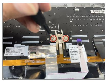
• Use the Phillips #0 screwdriver to remove the two 2.5 mm screws on the metal plate in the center of the keyboard.
