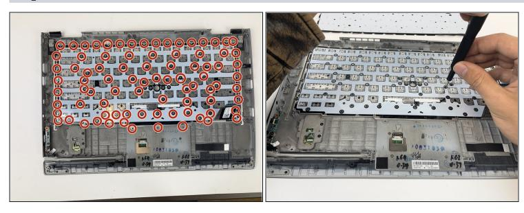
• Remove all the 2 mm screws from the back of the keyboard using a Phillips #000 screwdriver.
