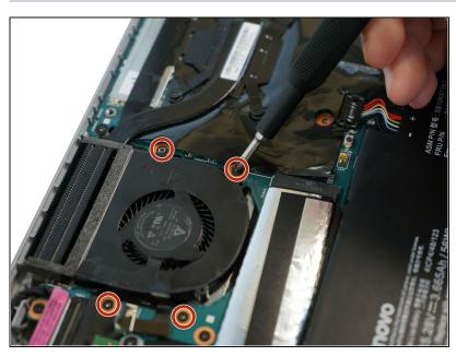
Using the Phillips #0 screwdriver, unscrew the four 4 mm screws directly next to the fan.
