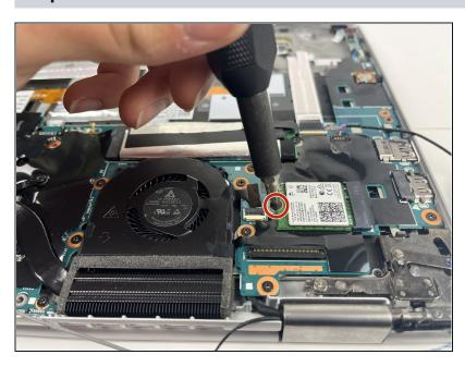
Remove the 3 mm screw from the Wi-Fi card using a Phillips #0 screwdriver.
