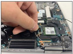
• Disconnect the gray and black coaxial cables from the Wi-Fi-Card using a spudger.
