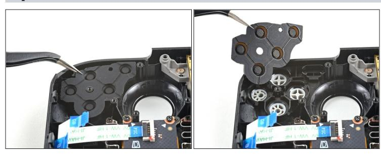
• Use a pair of tweezers to remove the action buttons and menu button membrane.
