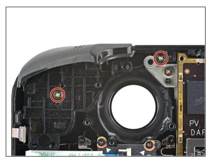
Use a Phillips driver to remove the two 5.2 mm screws securing the right bumper assembly.
