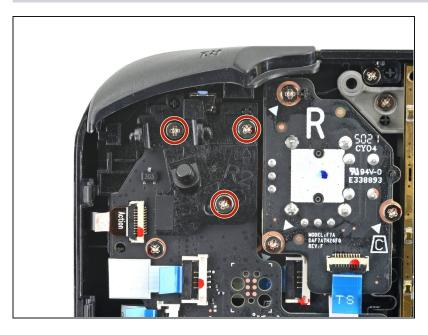
Use a Phillips driver to remove the three 5.2 mm screws securing the right trigger bracket.
