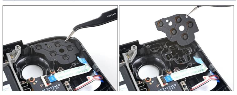
• Use a pair of <u>tweezers</u> to remove the D-pad membrane.
