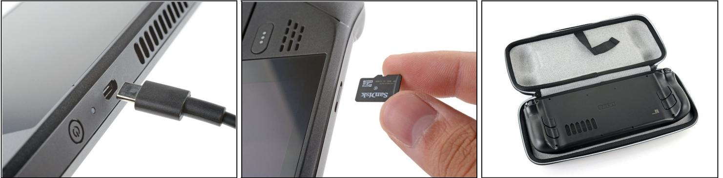
⚠ Turn on your Steam Deck and allow the battery to discharge below 25% before starting your repairs, as a charged lithium-ion polymer battery can be dangerous if accidentally punctured.
