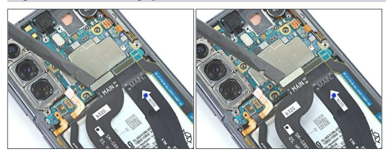
• Use the flat end of a spudger to pry up and disconnect the display cable's press connector.
