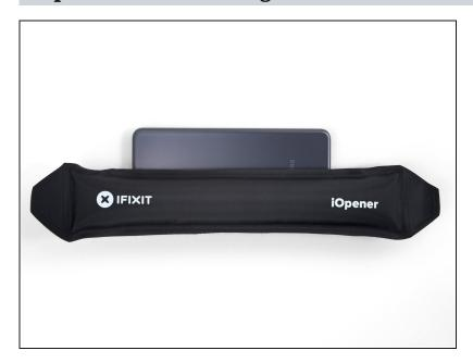
Apply a heated iOpener to the back cover's left edge for two minutes.
