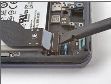
Use a spudger to pry up and disconnect the display cable's press connector near the bottom of the device.
