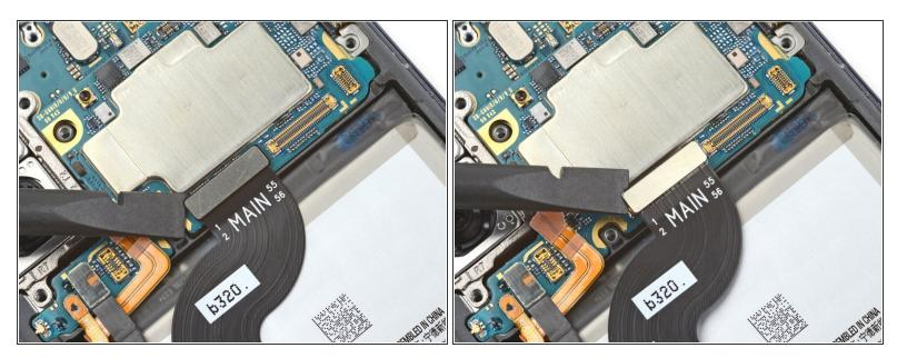
Use a spudger to pry up and disconnect the display cable's top press connector.
