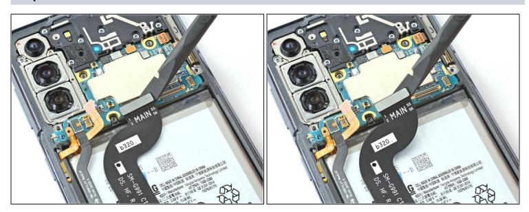
Use a spudger to pry up and disconnect the display cable's top press connector.
