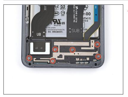
Use a Phillips screwdriver to remove the six 4 mm screws securing the loudspeaker to the frame.
