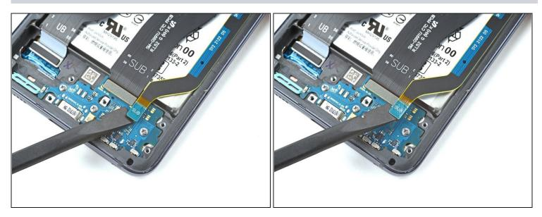
Use the flat end of a spudger to pry up and disconnect the secondary interconnect cable's press connector.
