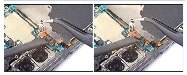
While still holding the motherboard bracket out of the way, use a spudger to pry up and disconnect the wireless charging coil's press connector.
