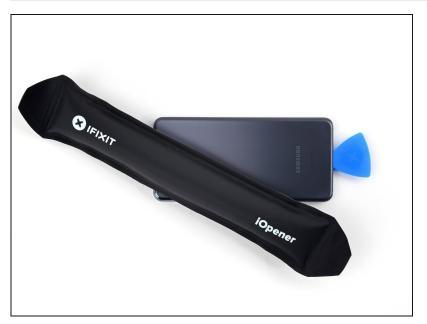
Heat an iOpener and apply it to the camera shell for two minutes.
