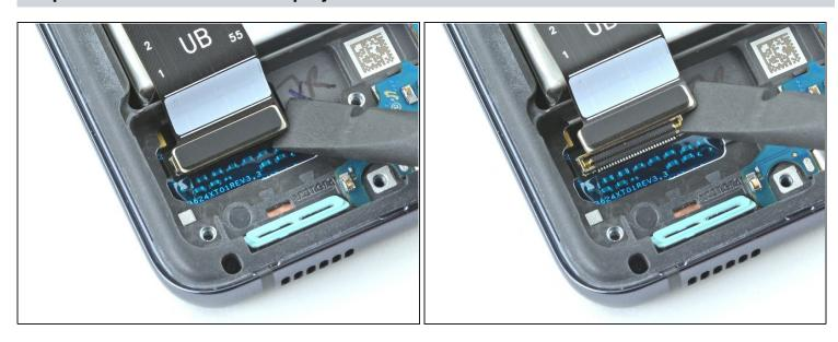
• Use a spudger to pry up and disconnect the display cable's bottom press connector.
