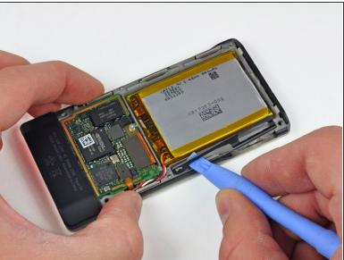
Use a Zune opening tool to gently lift the media button lever off the post cast into the inner chassis.
