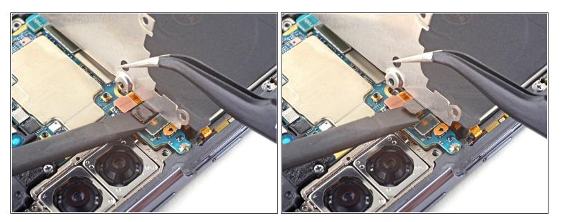
While still holding the motherboard bracket out of the way, use a spudger to pry up and disconnect the wireless charging coil's press connector.
