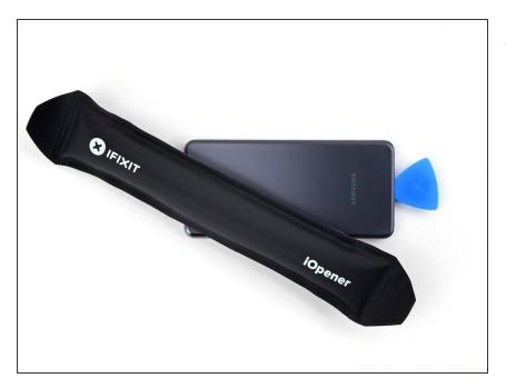
Heat an iOpener and apply it to the camera shell for two minutes.
