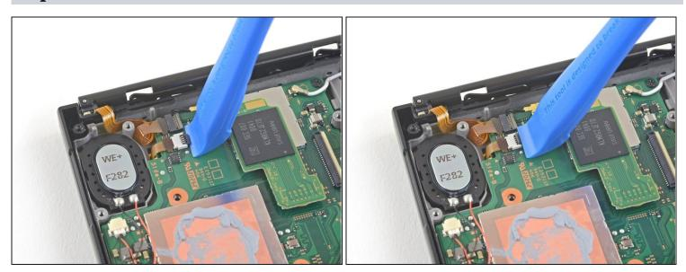
• Use an opening tool, spudger, or your fingernail to flip up the small, hinged locking flap on the smaller LCD ribbon cable <u>ZIF connector</u>.
