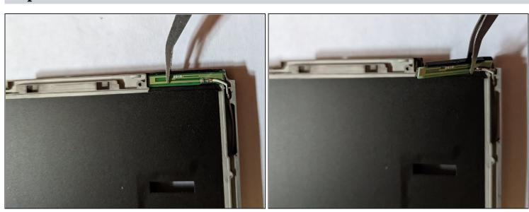
• The antenna is held in with light adhesive, so simply grasp it and pull up to release it.
