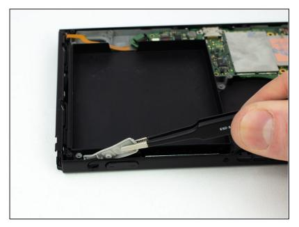
Pull the rubber conductive pad out with a pair of blunt nose tweezers.
