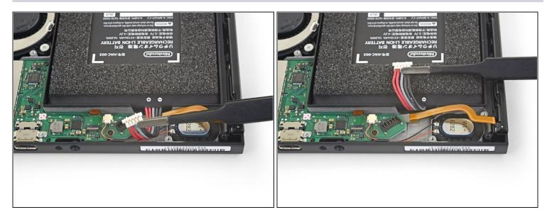
• Use your fingers or a pair of tweezers to lift the battery connector up and out of the way of the Joy Con rail's data cable.
