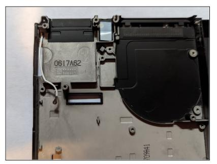
Verify the coax wire is free of any obstructions or routing inside the device.
