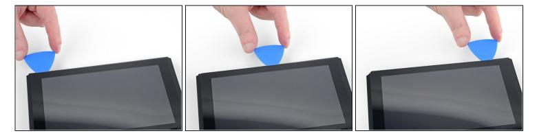
• Continue sliding the opening pick along the top edge of the screen to slice the adhesive.
