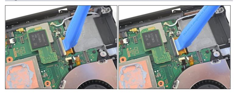
• Use an opening tool, spudger, or your fingernail to flip up the small, hinged locking flap on the LCD ribbon cable <u>ZIF connector</u>.
