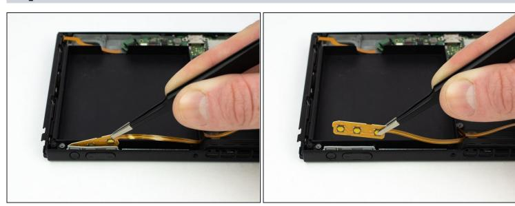
• Remove the power/volume board with a pair of blunt nose tweezers.
