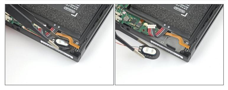
• Use your fingers or a pair of tweezers to carefully remove the speaker from the speaker well.
