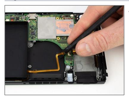
Use the flat end of a spudger to pry up the taped down power/volume ribbon cable.
