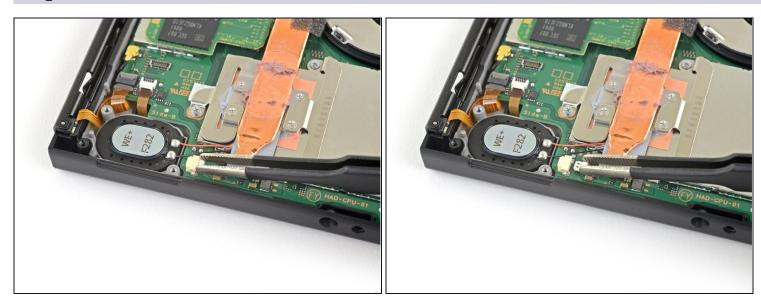
• Use your fingers or a pair of tweezers to pull the right speaker connector straight out of its socket on the motherboard.
