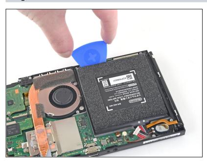
Continue sliding the opening pick deeper along the top edge of the battery, slicing more of the adhesive underneath.
