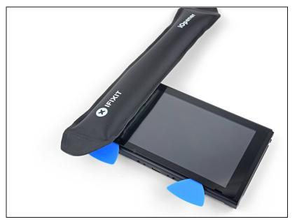
Heat the left edge of the screen for around two minutes to help soften the adhesive.
