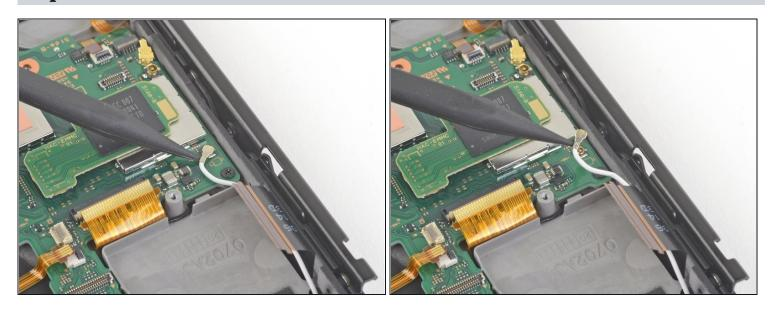
• Use the point of a spudger to pry up the white antenna cable straight up out of its socket on the motherboard.
