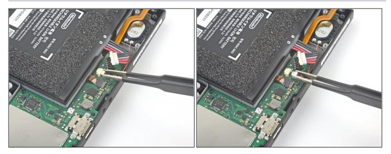
• Use your fingers or a pair of tweezers to pull the left speaker connector straight out of its socket on the motherboard.
