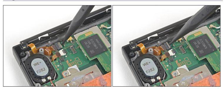
Use the point of a spudger, an opening tool, or your fingernail to flip up the small, hinged locking flap on the Joy Con sensor rail's data cable <u>ZIF connector</u>.
