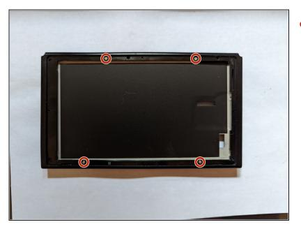
Remove the four screws securing the front frame to the midframe.
