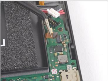
• Use a pair of tweezers to slide the Joy Con rail data cable straight out of its connector on the motherboard.
