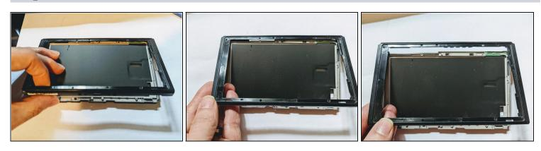
• Lift the front edge of the frame then slide the frame up toward the top of the display to remove it.
