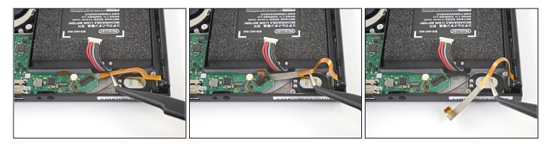
• Use your fingers or a pair of tweezers to lift the battery connector up and out of the way of the Joy Con rail's data cable.
