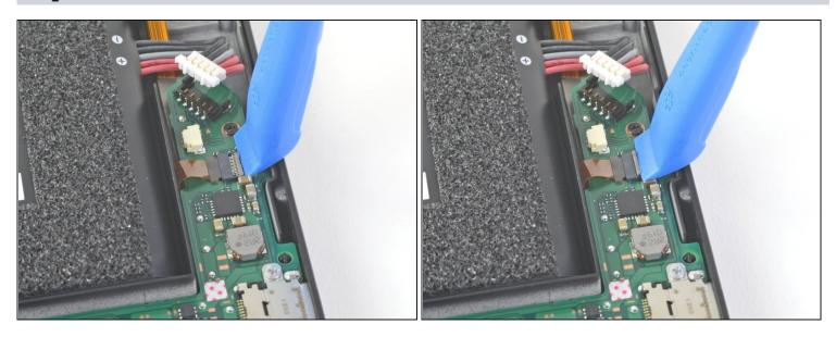
• Use an opening tool, spudger, or your fingernail to flip up the small, hinged locking flap on the Joy Con sensor rail data cable <u>ZIF connector</u>.
