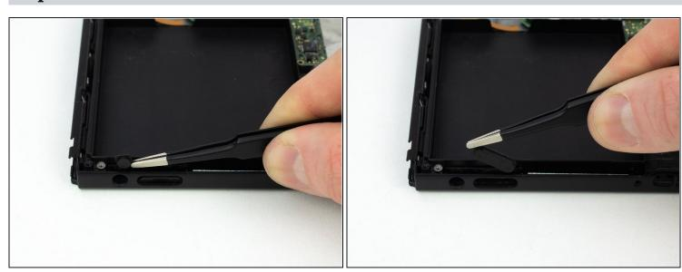
• Pull the power and volume buttons out with a pair of blunt nose tweezers.
