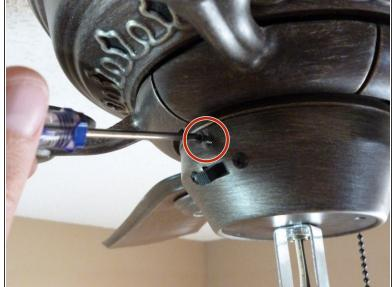
Replace the three 12 mm screws securing the lower switch housing to the upper switch housing with a Phillips #1 screwdriver.
