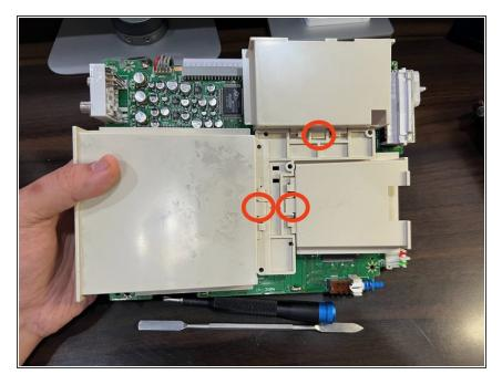
With the motherboard liberated, simple unsnap the three encircled clips of the expansion port bays.
