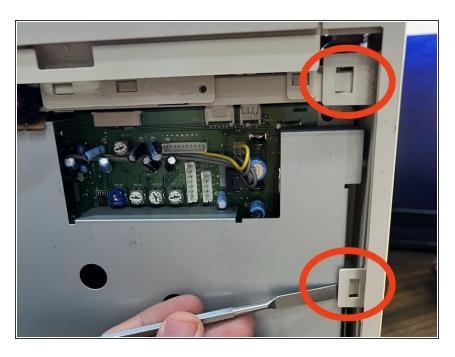
Remove the front panel attached by three clips on each side. The top two clips on the left are encircled in the picture.
