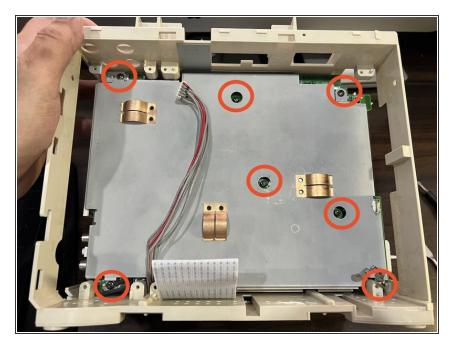
Remove the four corner screws, and the three long screws in the middle of the motherboard.
