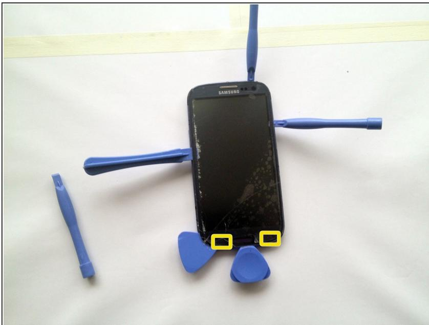
**⚠** When you start separating the screen, you need to start *from the top borders and work your way to the center*, ungluing the **whole screen** from top to bottom. Leave some opening tools in to prevent the glass from bonding again to the LCD.
