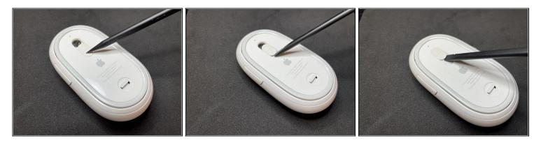
Slide the power switch to the off position or until it fully covers the optical sensor.
