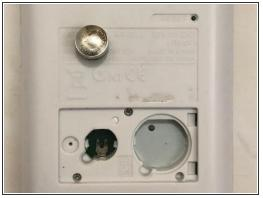
Place a spudger in the slot next to the battery and pry upwards to remove the battery.
