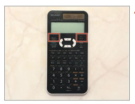
Press the 2nd F button and then the OFF button to power down the calculator.
