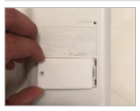
Remove the battery cover using two fingers.
