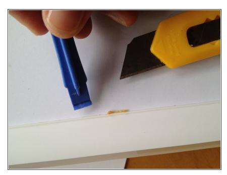
After the contact cement has dried, take out the small contact cement remnants from the board with a box cutter and a plastic tool (as to not damage the whiteboard)
