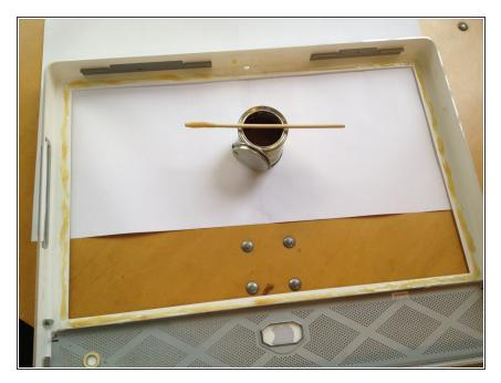
Apply contact cement to the inside borders of the front case. Leave to dry for about 5 minutes.
