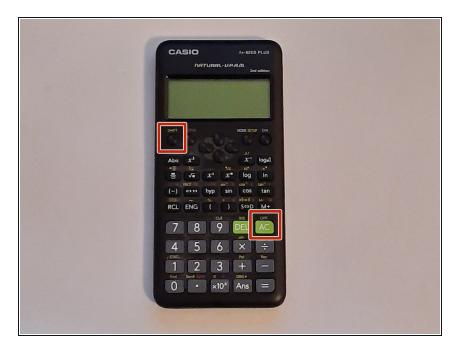
Turn off the calculator before you begin by pressing the shift button first and at the same time press the AC button.
