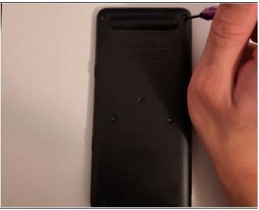
Turn the calculator over and using the Phillips #1 screwdriver, remove six 5mm from the back cover.
