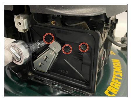
Use the socket wrench and put the 5/16" inch hex bit on to remove the three 20 mm bolts located behind the air filter.
