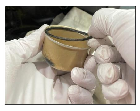
Remove the O-Ring from the carburetor tank and replace it with a new one. You are ready to reassemble your lawnmower! To reassemble your device, follow these instructions in reverse order.
