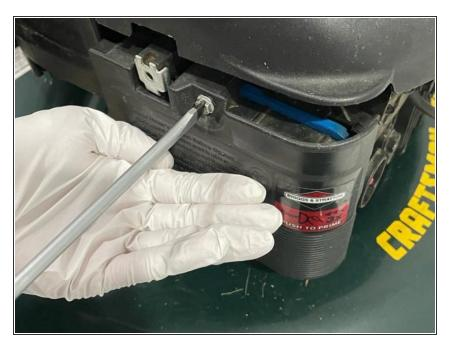
Use a flathead screwdriver and remove the 40 mm screw that secures the air filter and the case to the lawn mower.
