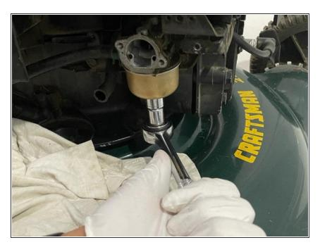
Use the socket wrench with a ½" inch hex bit to remove the 11 mm screw on the bottom of the tank.
