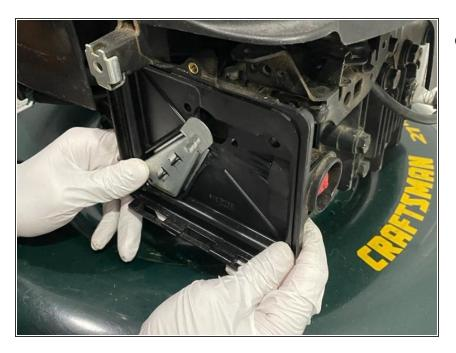
Pull the plastic backing off which will expose the carburetor.
