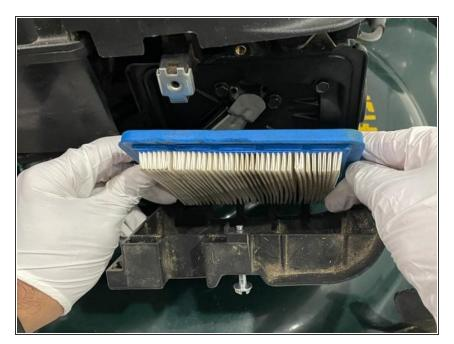
Carefully remove the air filter and set it aside.
