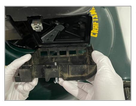
Slowly remove the air filter case from the hinges by tilting it slightly and pulling it out.
