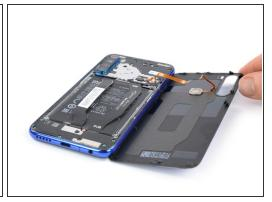
Carefully fold the rear glass to the right side of the phone assembly like you'd open the back cover
