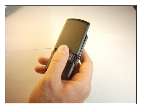
Push from indentation and slide battery cover away from phone to remove battery cover.
