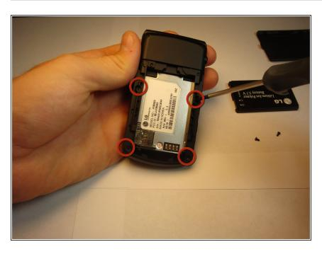
Using a philips screwdriver, unscrew all 4 screws along the edge of the phone
