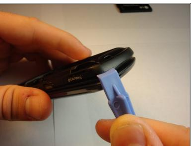
Using your plastic pry tool, insert the tool between the phone's keypad cover and back cover and gently pry apart.
