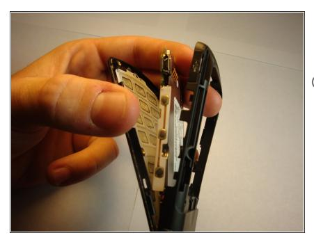
Once the covers have been separated the motherboard will be visible. Do not separate the two covers completely. The covers will be held together by a screw on the axis of the phone.
