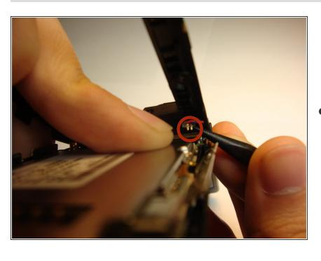
(Ignore this step if the screen display connector is already separated from the motherboard) Using the spudger, place the pointy end between the plastic end of the wire and the motherboard and lift/push wire from the motherboard socket. You should see two golden pins protruding from the plastic.
