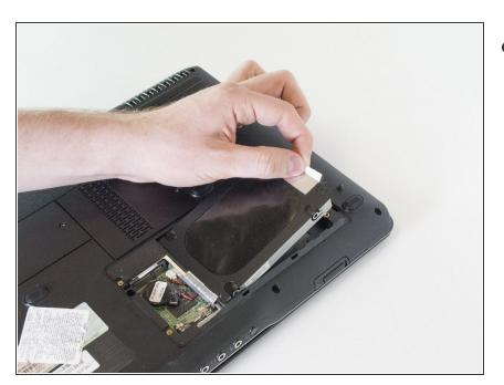
• Lift up this internal panel using the plastic white tab and set it aside.
